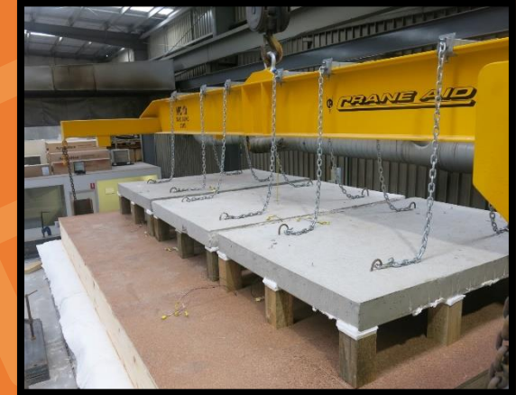
The timber floor was point loaded with 1.7 tonne of concrete
