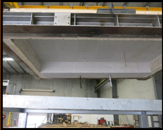
Bulkhead and ceiling specimen buildup complete
