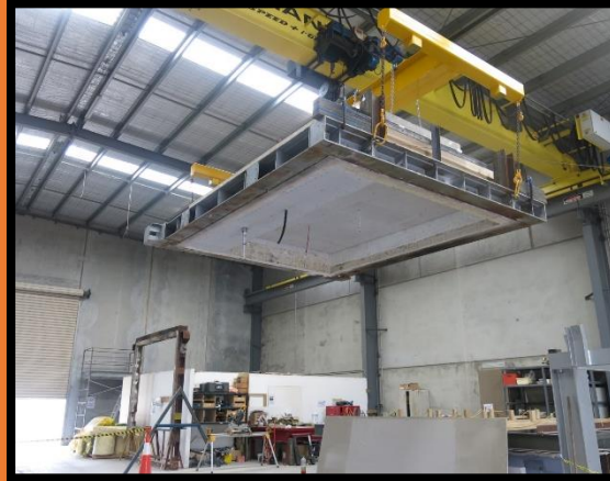
Specimen being lifted onto the furnace
