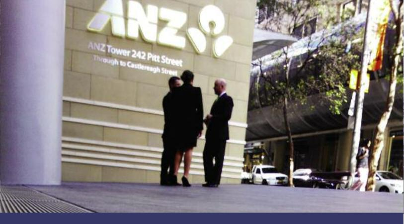
10mm wide drainage grate slots are a reasonable compromise between protecting heels and canes, and collecting surface water . . . you can only ever design for 98% of the population.
