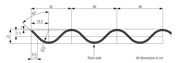
Silent Gliss 6010 - Gliding channel 5.4 mm → only applicable with glider SG 6082.
