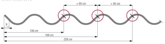
Further symmetric cutting measurements: 288 cm, 348 cm, 408 cm, 468 cm
