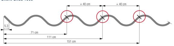
Further symmetric cutting measurements: 191 cm, 231 cm, 271 cm, 311 cm, 351 cm, 391 cm, 431 cm, 471 cm
