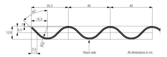
Silent Gliss 6465 - Gliding channel 5.4 mm  $\rightarrow$  only applicable with glider SG 6082.
