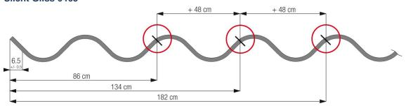
Further symmetric cutting measurements: 230 cm, 278 cm, 326 cm, 374 cm, 422 cm, 470 cm
