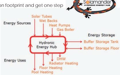
The system can prioritise renewable energy sources over non renewable energy sources to ensure minimal energy wastage. The prioritisation of renewable energy sources like solar power reduces the energy costs associated with domestic hot water and other heating related utility bills.
